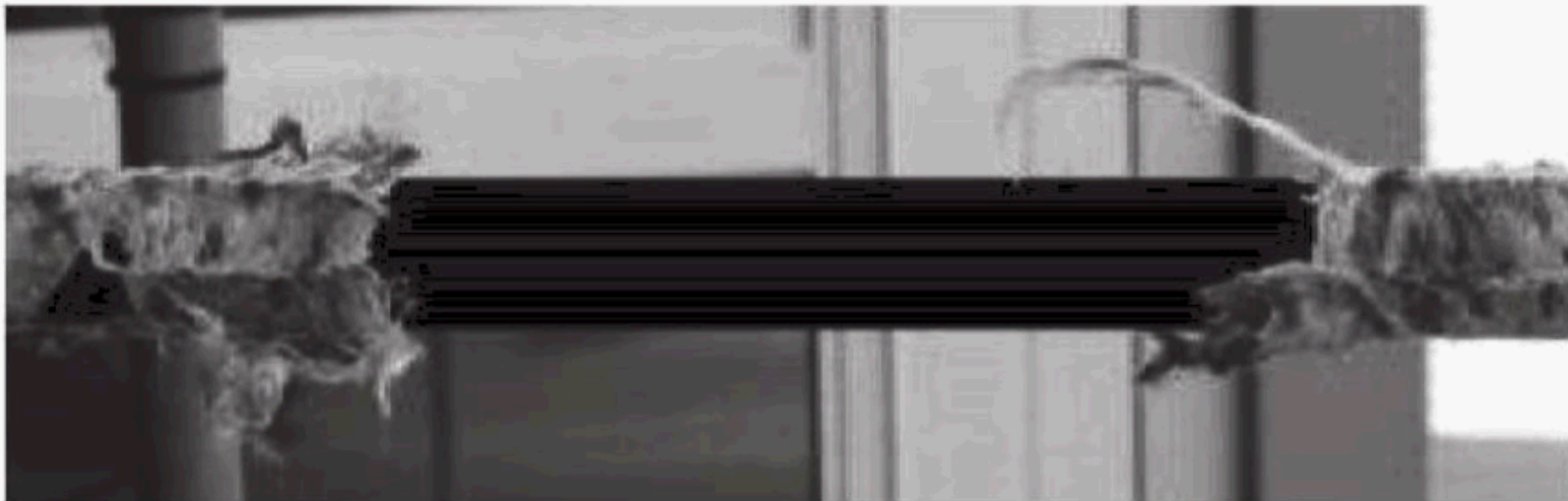
Figure 30-2.8.2-7 Broken Jackets
