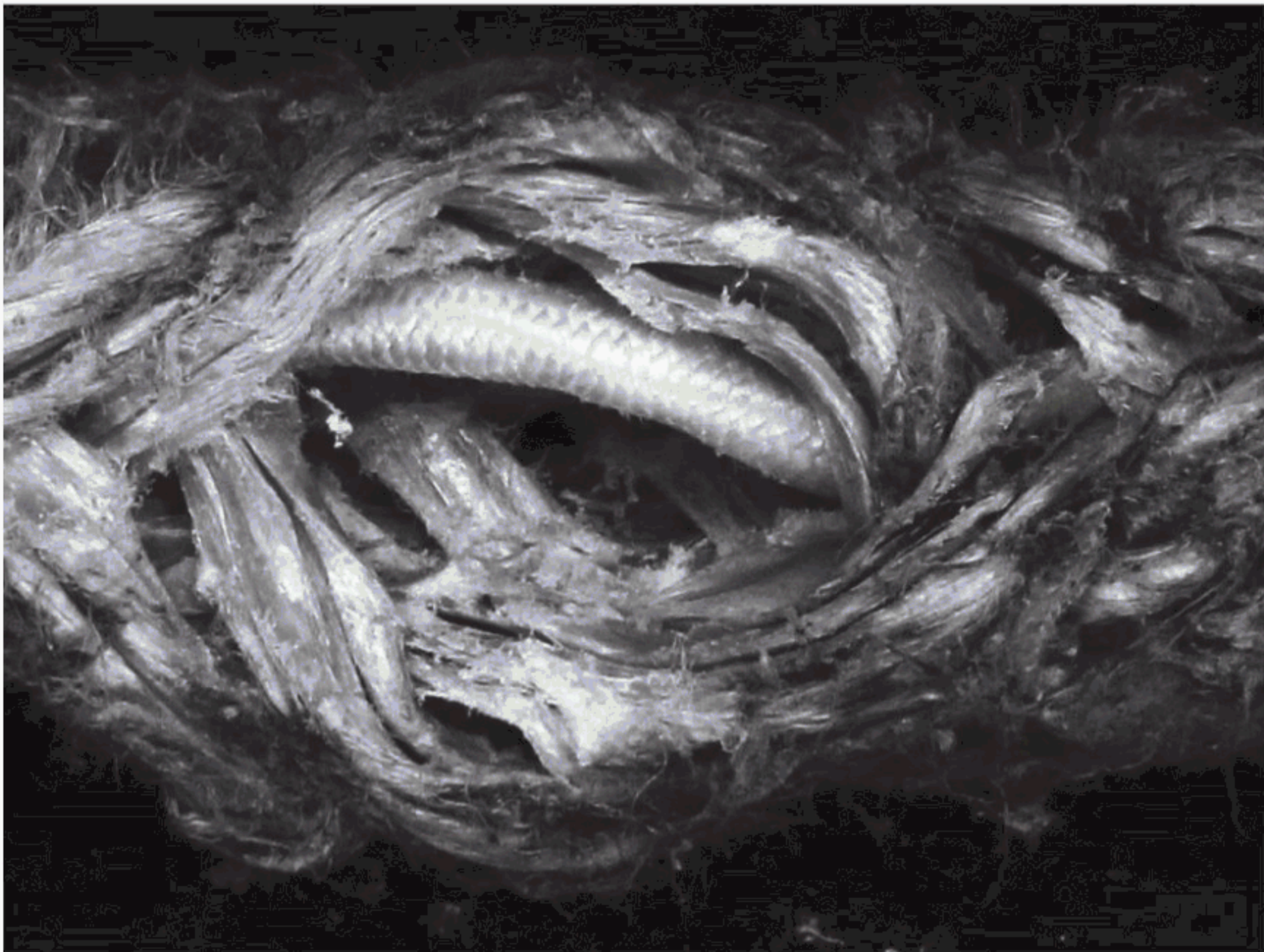
Figure 30-2.8.2-3 Damage Inside the Rope
