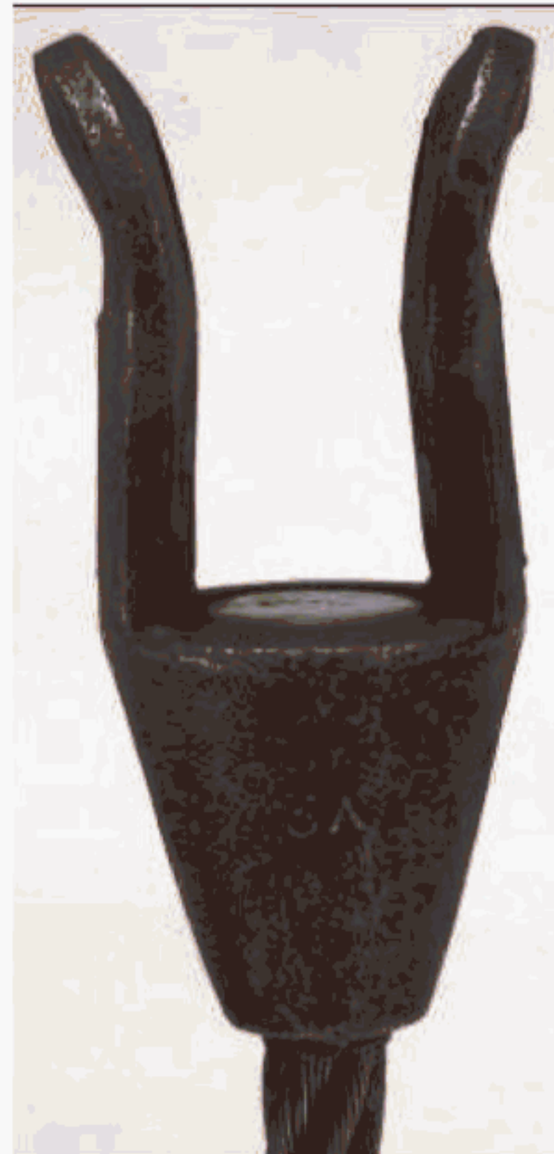
Figure 30-1.8.2-9 Damaged End Terminations
