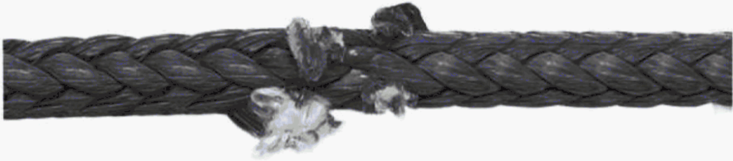
Figure 30-2.8.2-1 Cuts, Gouges, and Yarn Material Breakage
