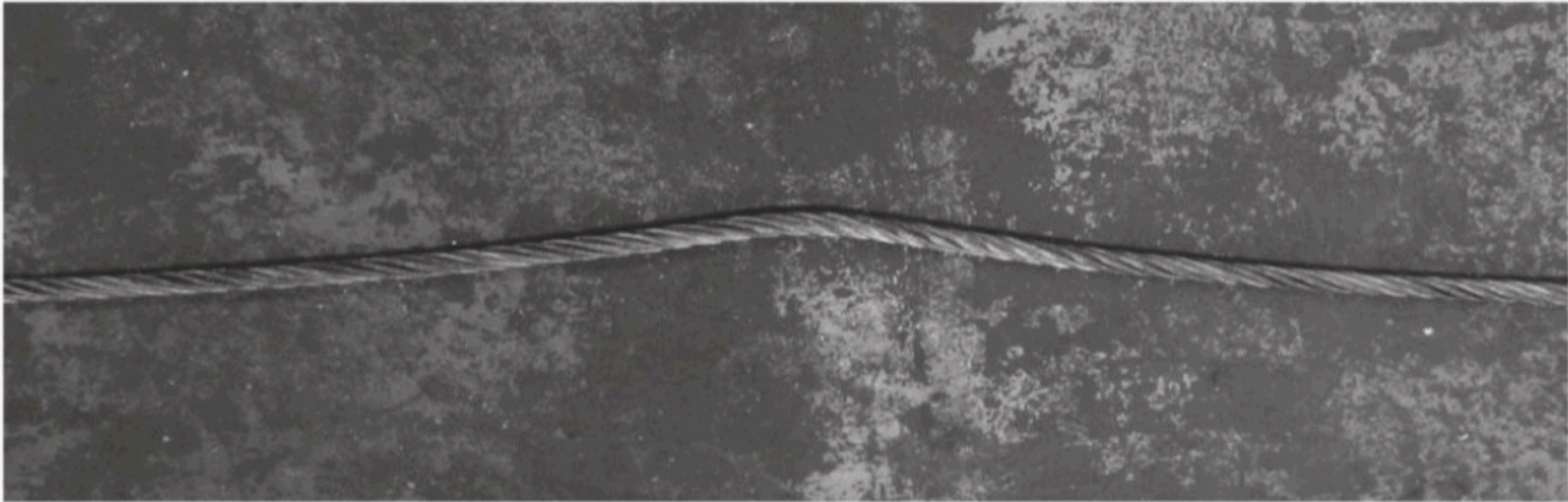
Figure 30-1.8.2-2 Distortion of Rope Structure — Dogleg
