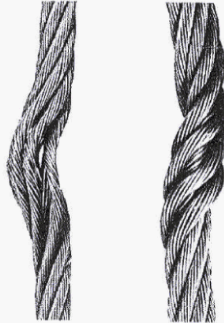
Figure 30-1.8.2-1 Distortion of Rope Structure — Kink
