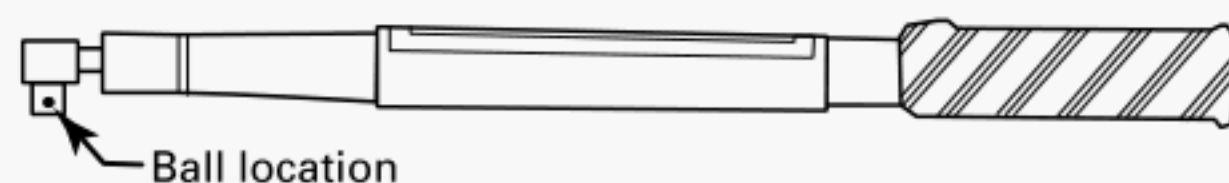
Figure 5.7.1-1 Drive Ball Location
