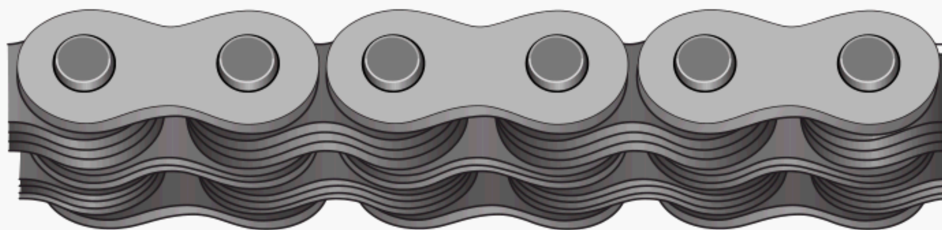
FIG. 1 ASSEMBLY SHOWING 3 × 4 LACING
