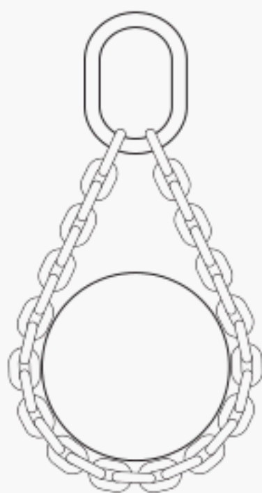
(c) Single-Basket Sling and Hitch
